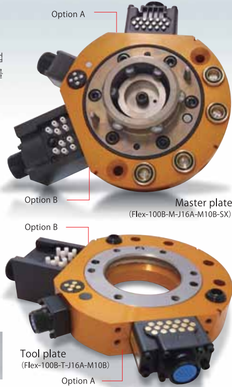
Master plate Attachments • 6 bolts (M8×55) • Stepped parallel pin × 1 ※ Seal plate, O-ring and screws are pre-assembled.
