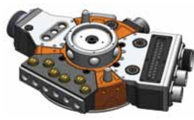
5 Model for exchanging spot welding guns and for handring hands or jigs.
