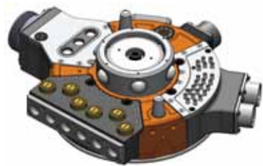
1 Model for spot welding gun exchange.
